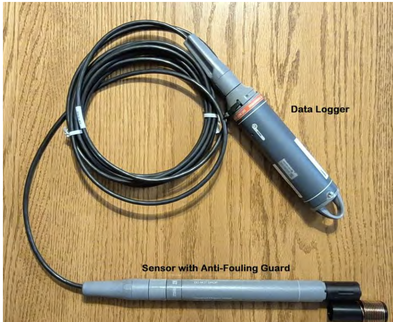
Onset/HOBO DO Sensor and Logger (sampling interval= 20 sec)
