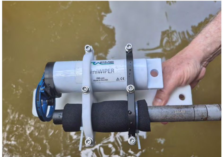
DO Sensor Integrated w/ PME Wiper Module (cleaned off detector 4x/day)
