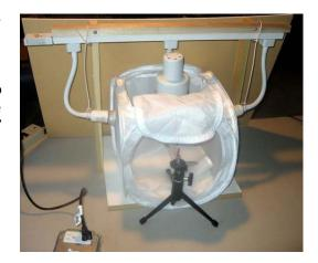
**Lighting details:** With the diffuser removed, you can see that the lights are positioned to direct light on the fly. To keep the goosenecks from gradually straightening, a couple of pieces of #12 gauge electrical wire are wrapped around these fixtures and the track to hold the position of the lights.
